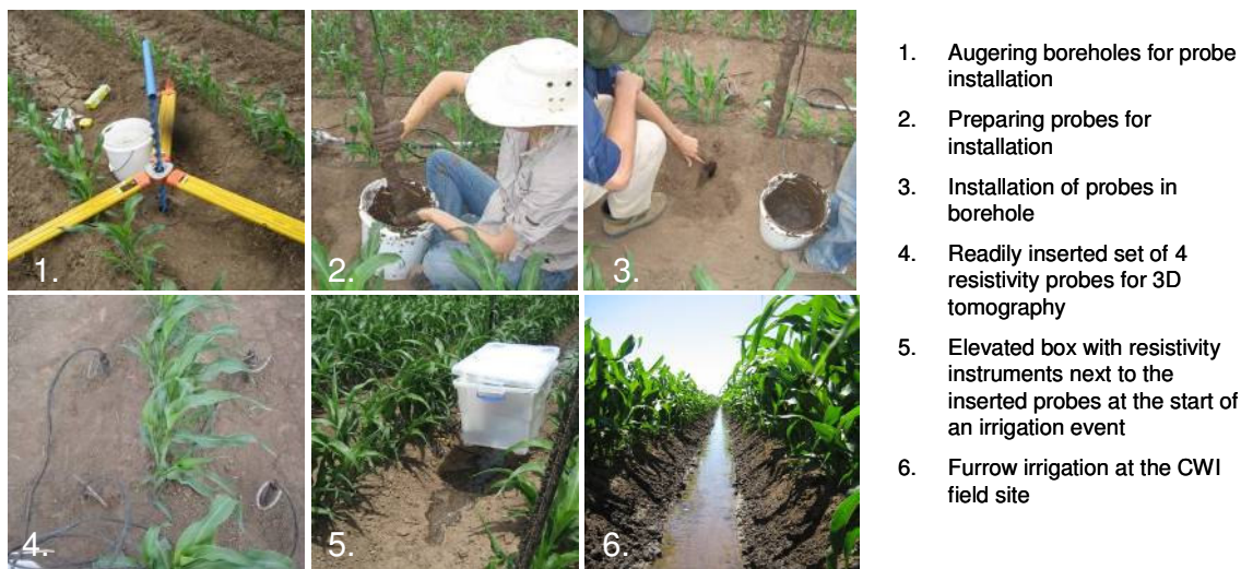
Figure 5: installation and operation of 3D borehole tomography probes at the CWI field site
