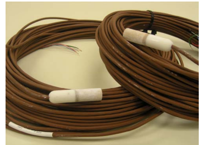
Heat Dissipation Sensor (0.1 to -35,000 m; \pm 1 m) QAd2331Bx
