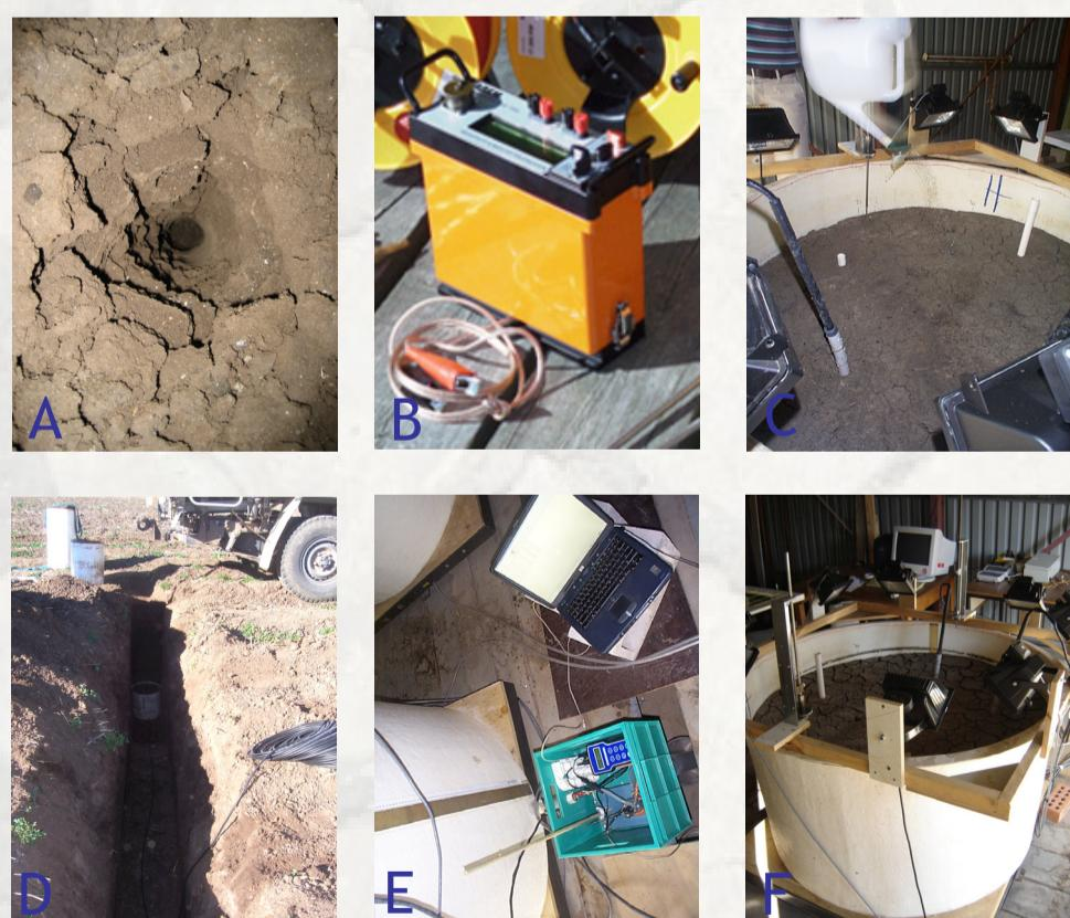
A: soil core in dry cracked soil B: ABEM resistivity meter for electrical resistivity tomography C: Tracer application on soil column D: Lysimeter installation in the field E: EC monitoring and collection of effluent from soil column F: light setup for time lab surface images
