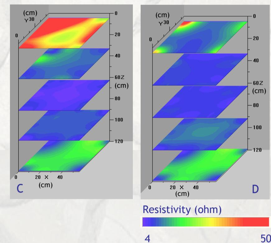
A-B: Sorghum field before and during flood irrigation C-D Resistivity distribution in clay soil before and after flood irrigation (units on axis are cm)
