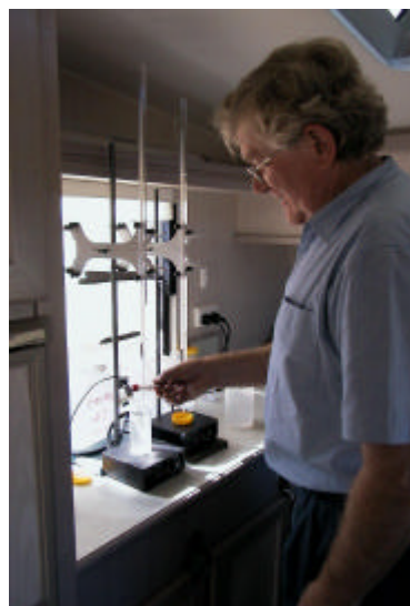
Figure 4.23: Field Titration For Unstable Parameters
