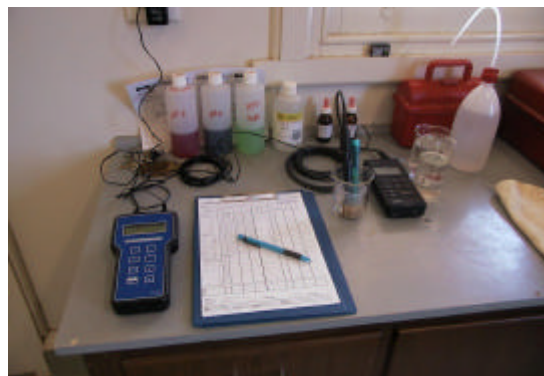
Figure 4.14: Measurement of pH and EC From 1:5 Aqueous Extract
