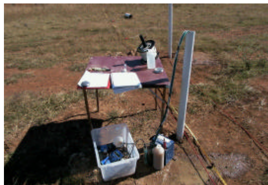
Figure 4.20: Pumping Shallow Bores With Amazon Pump, Measurement of Unstable Parameters, and Sample Collection
