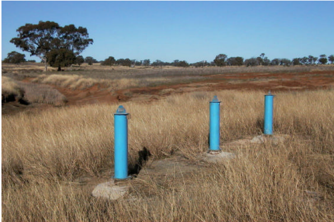
Figure 4.6: Nested Monitoring Bore Site GW96128
