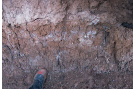
Figure 5.16: Columnar Shrinkage Cracks and Salt Efflorescence on Surface of Unit Two
