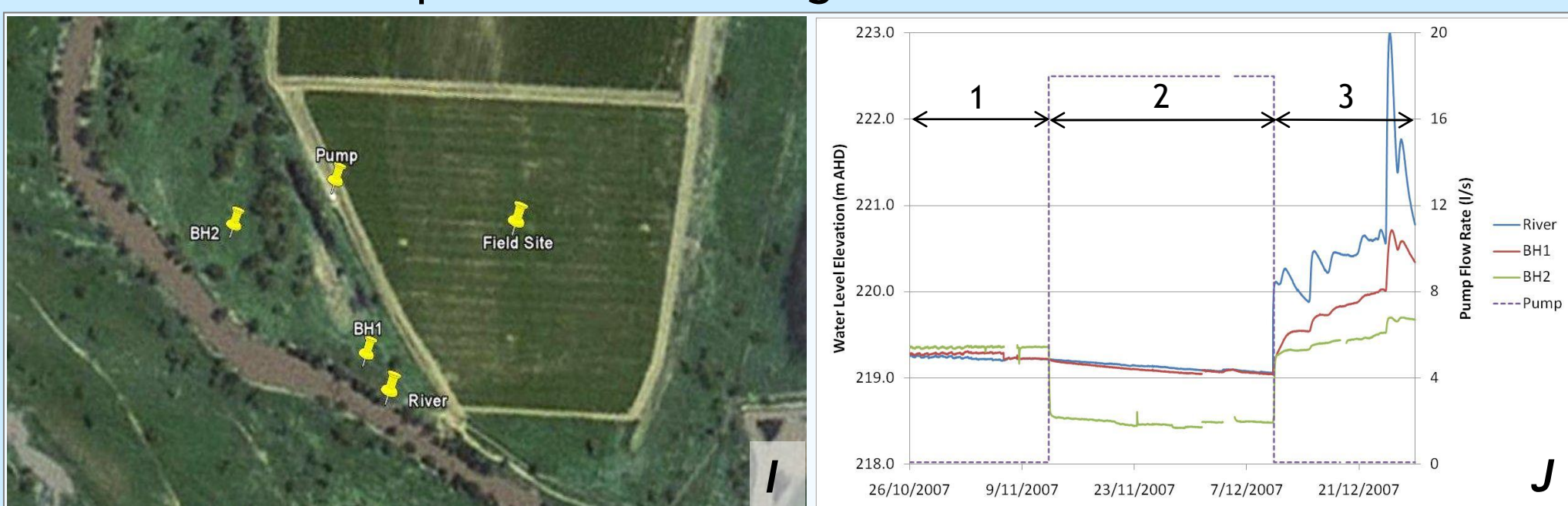
I: Image of field site showing location of river stage monitoring and boreholes. J: Hydrographs covering three periods: (1) non-pumping and non-flooding, (2) pumping, (3) flooding.
