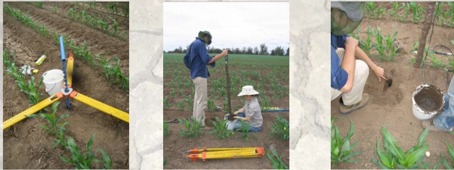
Installation of resistivity probes (1-2.11.2007)
