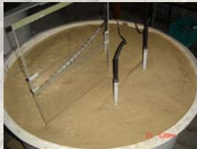
Lab study in sand filled lysimeter
