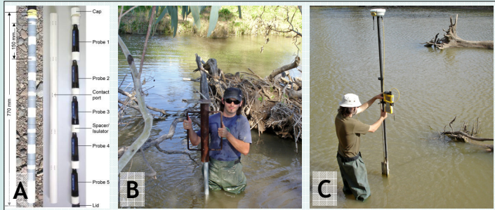
A: Dimensions of temperature array. B: Installation in the streambed. C: DGPS positioning.
